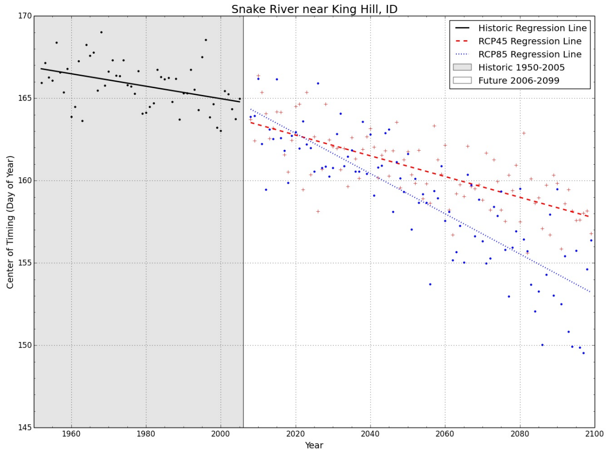
Figure C.10 Center of timing for Snake River at King Hill, showing shaded historic (1950-2005) and future (2006-2099)
